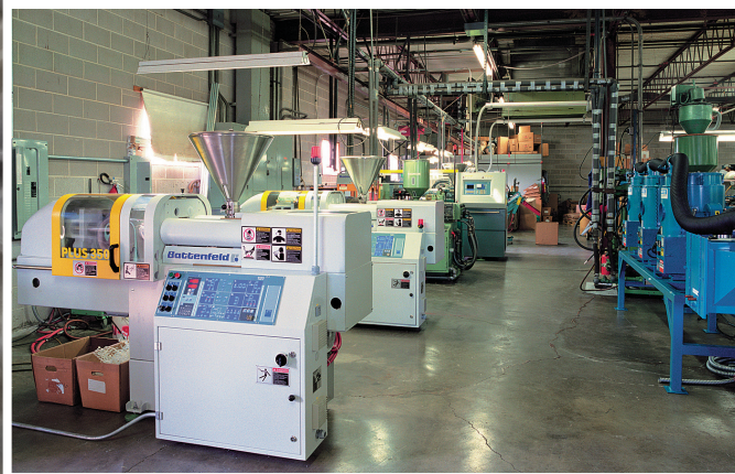
On these molding machines, DU-BRO produces injection-molded plastics with fresh resin to ensure maximum durability.
