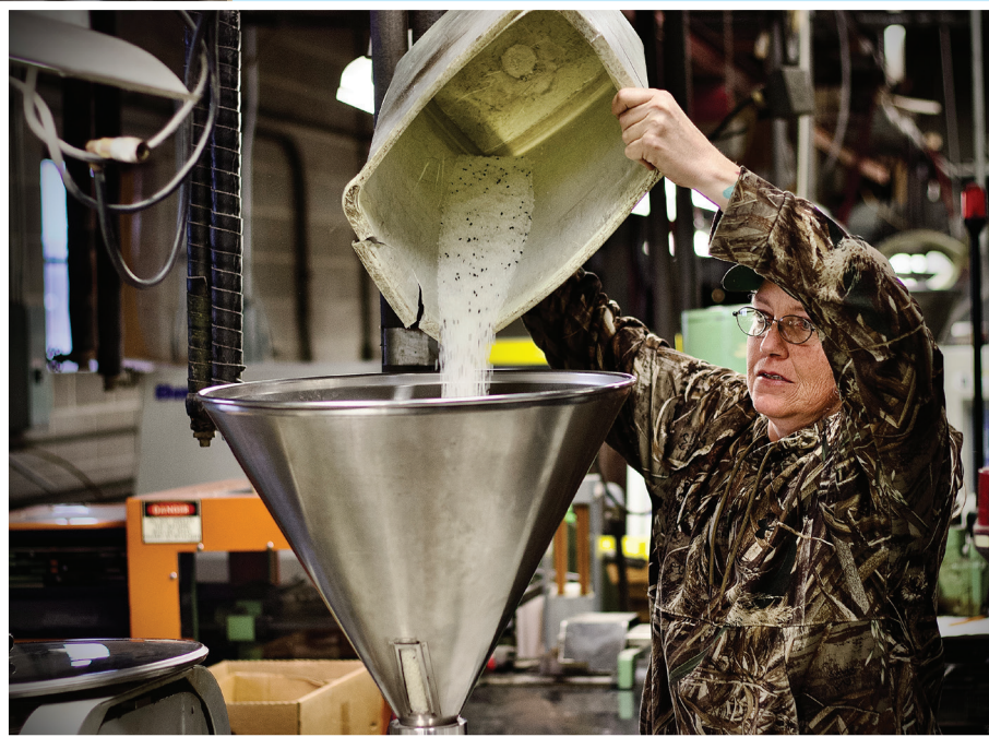
A worker loads a fresh resin into the hopper of an injection molding machine.
